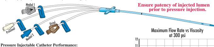
For pressure injection equipment limited to 300 psi, the following chart (graph) shows the maximum achievable flow rates as a function of viscosity.
